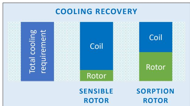
**Figure 1.** Reducing the capacity of the cooling coil due to the use of sensible and sorption rotors.
