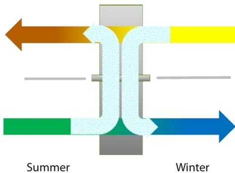
In summer, when the humidity is higher, moisture is removed from the outdoor air and transferred to the exhaust air. In winter, moisture is transferred from extract to supply.
