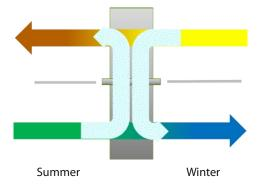
In summer, when the humidity is higher, moisture is removed from the outdoor air and transferred to the exhaust air. In winter, moisture is transferred from extract to supply.
