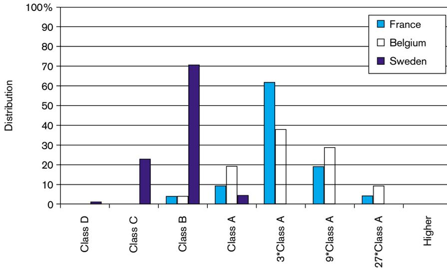
**FIGURE 13.** Distribution of the different airtightness classes based on measurements carried out in 21 systems in Belgium, 21 Systems in France and 69 systems in Sweden. The bars represent the relative number of systems fulfilling the requirements for the specified airtightness class.
