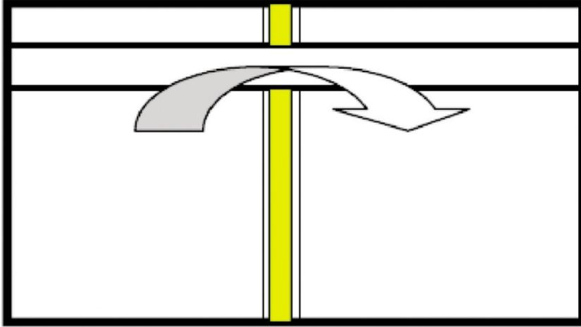
**FIGURE 6.** Crosstalk between two rooms via ducting.
