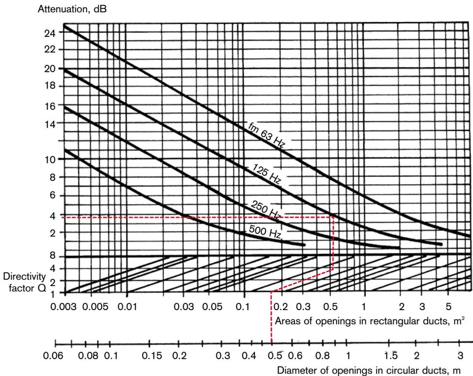
**FIGURE 5.** Attenuation in terminal devices and duct openings. The dashed line illustrates the following case: Directivity factor,  $Q = 4$  and the duct diameter = 0.5 m. Attenuation at a frequency of 125 Hz will be 4 dB.
