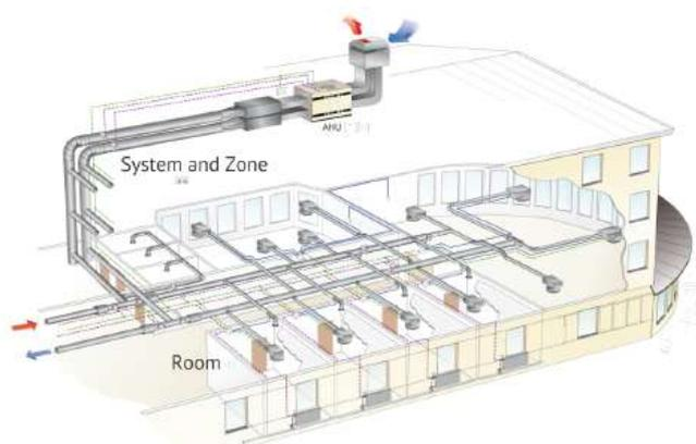
**Figure 1: DCV System technology – zone and system level along with room levels**
