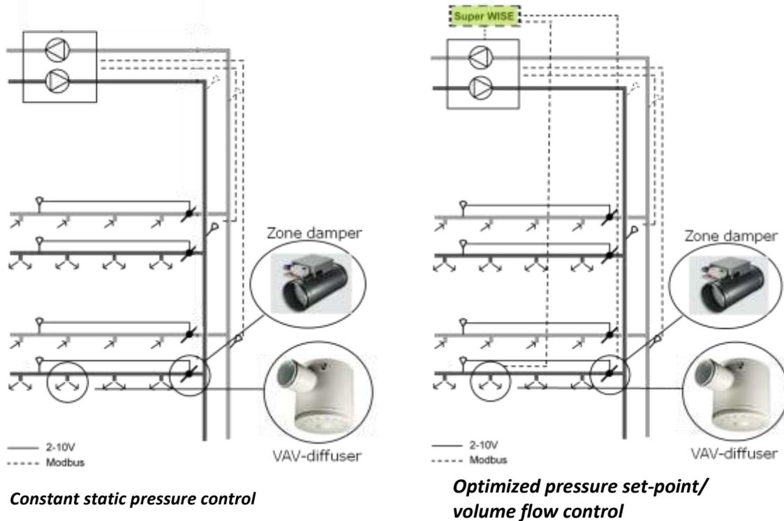
**Figure 2: Pressure control and air flow control schematics**
