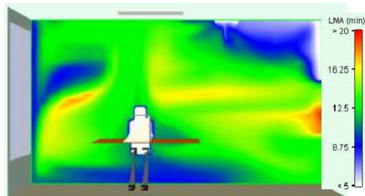
Figure 2.8 Typical age of the air in a cell office (LMA = Local Mean Average in minutes)
