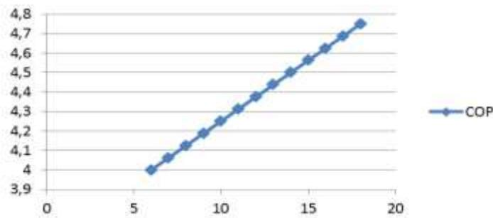
Figure 1.2 Chillers COP v water supply temp (deg C)
