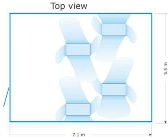
Figure 2.11 Top view air pattern in the test, created by guide fins to avoid draught.
