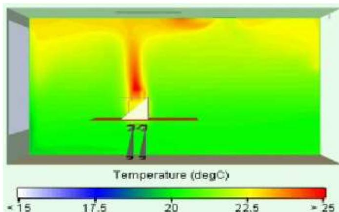
Figure 2.7 Typical air temperatures in a cell office
