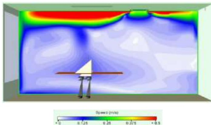
Figure 2.6 Typical air velocities in a cell office.
