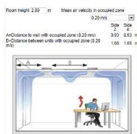
Secondly the positioning of chilled beams should be considered to avoid risk of draught. Depending on the nozzle pressure, airflow and capacity chilled beams should have a minimum distance between the units and also to walls and/or other affecting obstacles. Most manufacturers have software available to support guidelines of positioning (figure 2.5).
