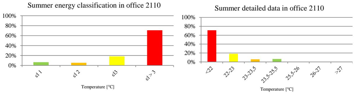
Figure 10. Detailed analysis of energy classification in office area in summer period (total and split in temperature ranges).
