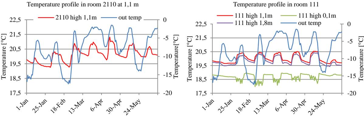
Figure 4. Indoor and outdoor temperature weekly profiles at office room 2110 and packing area 111 (temperature stratification).
