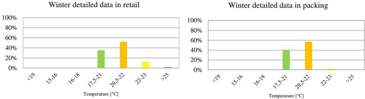
Figure 9. Detailed energy classification for retail and packing areas in winter period (total and split in temperature ranges).
