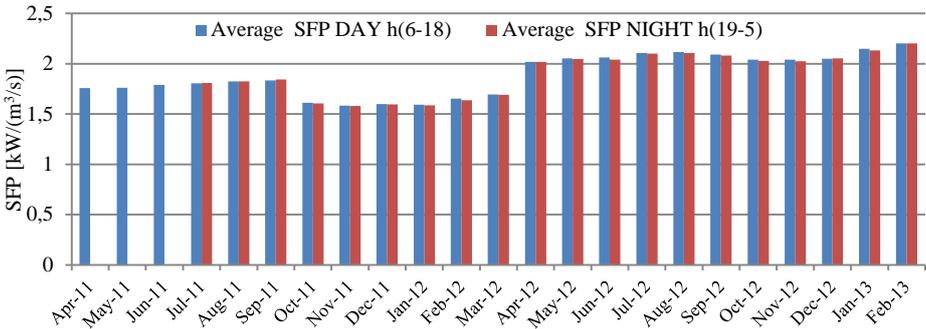
Figure 3. Monthly average of specific fan power (SPF, kW/(m³/s)) in day/night modes.
