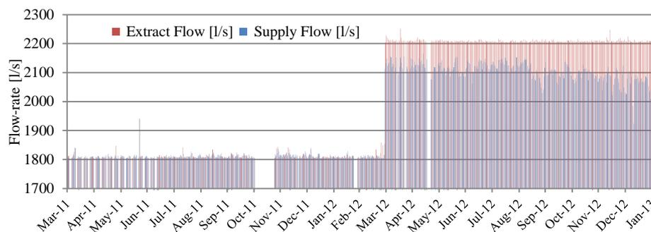
Figure 2. Extract and supply airflow values for TA/FA2 (missing data and increase of airflow).
