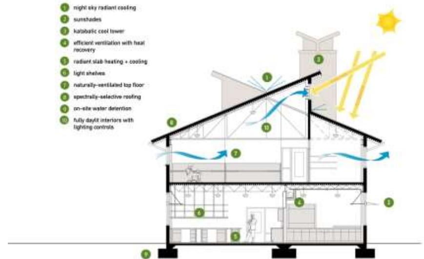
Let geometry, orientation and façade design solve solar problems (not air-conditioning)
