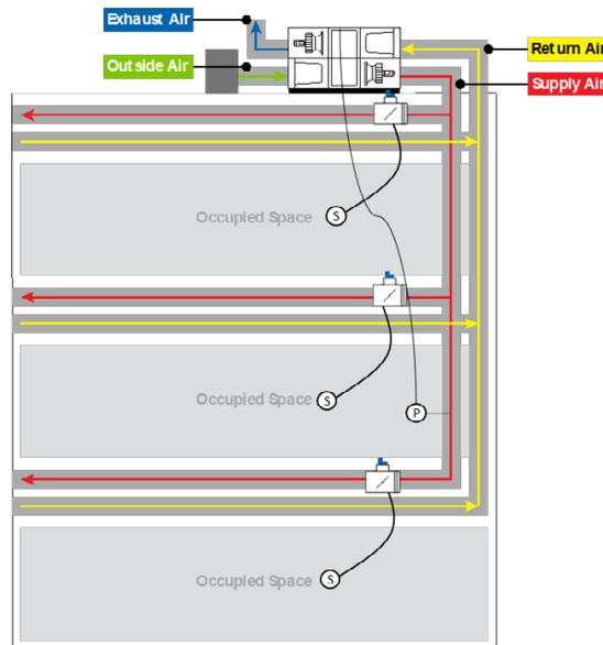
**Figure 7: Ventilation system with Zone Airflow Control**
