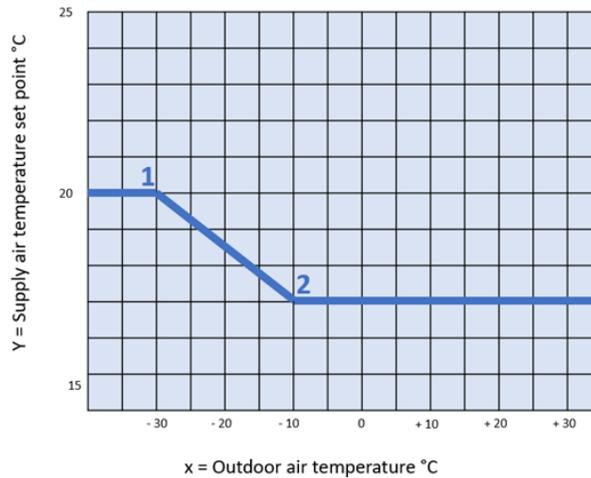
**Figure 6: Ventilation Supply Air Temperature Reset**
